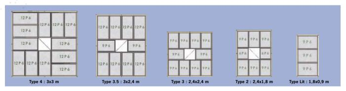
The type 4 CamHOSP2 modular ceiling with an operational surface of around 9 m2 for class ISO 5 to ISO 7 is ideally suited for major operations (for example, orthopaedic or cardiac surgery). It also provides a comfortable working environment for the surgical team.
